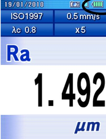
The screenshot shows the main display of the SJ-210. At the top, it displays the date '19/01/2010', a camera icon, and a battery level icon (a battery symbol with four segments, the rightmost being green). Below this, it shows 'ISO1997' and '0.5 mm/s' in the first row, and 'λc 0.8' and 'x5' in the second row. The measurement result 'Ra' is shown in large blue letters, with the value '1.492' below it, followed by the unit 'μm'.
